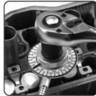
Loosening & tightening the screw to zero the gauge
