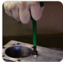
4. Screw coil into casting
