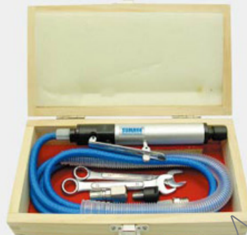
ST-3360LA 1/8" Industrial ST-3360LMA 3mm Micro Air Grinder (35,000r.p.m.)
