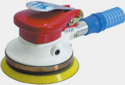
ST-7724 W/6" Velcro Pad ST-7724S W/6" Stick Pad Air Self Vacuuming Dust Free D/A Sander (10,000 rpm)
