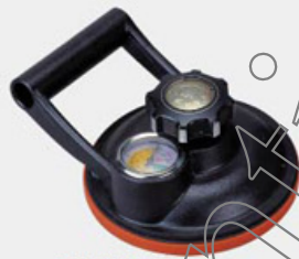
SC-9601HA Heavy Duty Suction Cup *The vacuum is produced by pressing the lever down.
