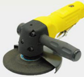
ST-P7736 100° 4" Air Grinder (M10x1.5 spindle) ST-P7736A 100° 4-1/2" Air Grinder (5/8x11 UNC spindle) ST-P7737, ST-P7737B 100° 5" Air Grinder (5/8x11 UNC spindle) Speed: 10,000 rpm ** W/O Grinding Disc
