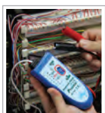
DC level testing function
