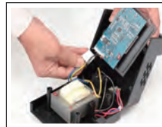
Modular design for easy repair (only for SS-207)
