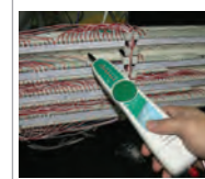
Locates and isolates cables quickly and easily
