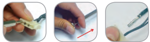
Put the pin extractor into housing Push the plunger of pin extractor Extract the pin
