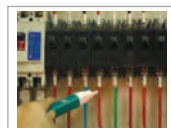
Detects AC voltage from 90 to 1000 VAC
