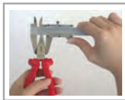
Outside diameter measurement
