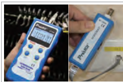
Verify LAN cable condition
